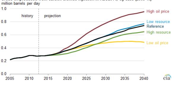
Crude oil produced from carbon dioxide injection in AEO2014, by case (2005-40)
